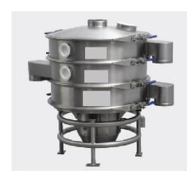
Rubber mounted suspension without spring – Acceptable.
